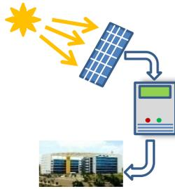
**With Battery Storage:** All the generated electricity is stored in battery bank and used either continuously or as backup when there is no supply from State electricity agency.
